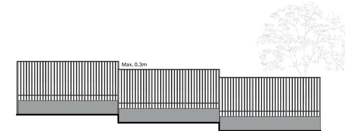
In case of level difference across elevation, the maximum stepping should be 0.3m
