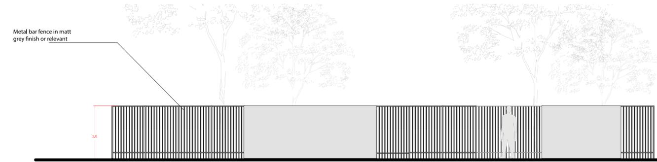
Figure 1.2 External Peripheral Boundary Elevation
