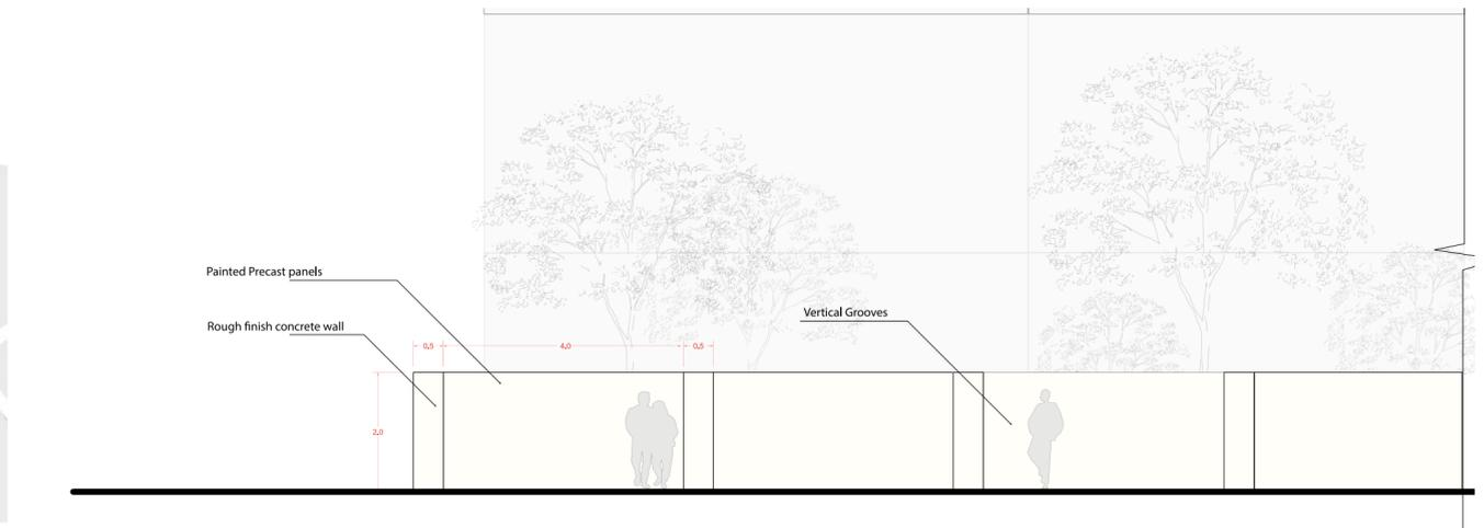
Figure 1.4 Boundary Type 1 Elevation
