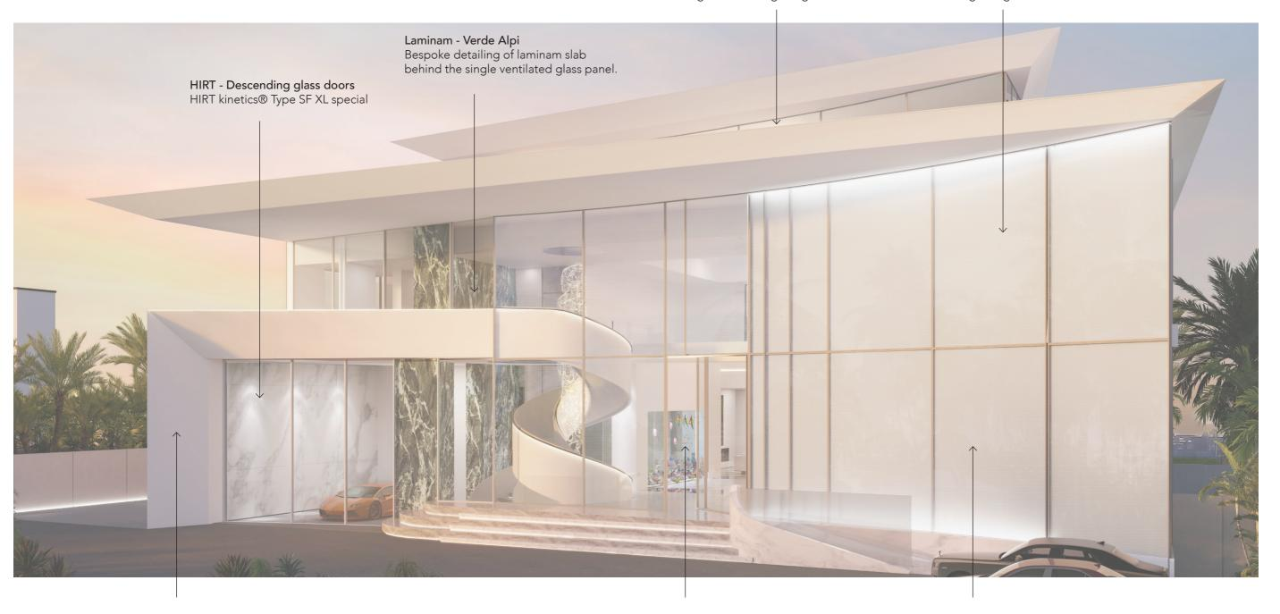
Caparol ETICS - Capatec system External Insulation Finish System in a Capastructure for White seamless finish. Vitrocsa TH+ - Pivot
